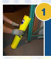
Tilt the Rack Armour® guard forward so that the bottom of the unit is approximately 300mm clear of the upright and hold at an angle of 45 degrees.
